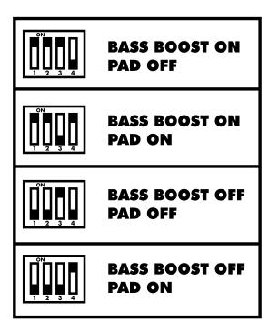
Depending on how you are using the Cortado MkIII, controlling how much "low end" you pick up is oftentimes very important for preventing the audio from sounding muddied. We have found that when the Cortado is being used with other microphones or in a mix of other audio sources, when the bass boost is OFF the sounds picked up by the Cortado are often much clearer and more distinct in the mix.
