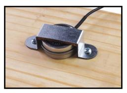
Double sided tape is a great option for permanently mounting the sensor to smooth surfaces. For capturing the fullest bandwidth, use thin double sided tape with very strong adhesive properties, such as the tape disc provided in the mounting accessory kit. Foam-type tapes will behave as a mechanical filter, tuning out certain frequencies. Sometimes, this may be just what you need for capturing a particular sound. Feel free to experiment.
