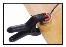
Mounting straps for the Cortado MkIII sensor (included in the optional accessory kit) are perfect for permanently mounting the sensor to a wooden surface, such as the underside of a basketball court or tap dance floor. When using a mounting strap make sure to place the sensor in the very middle of the bracket, so that neither side of the strap touches the side of the sensor head. Use the supplied screws to attach the strap to the vibrating surface.
